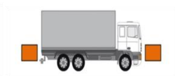
Packaged hazardous substance
